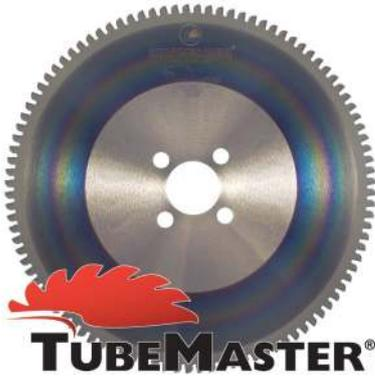
TubeMaster saw blades have especially been designed for orbital flying cut-off applications on tube mills. Key features of this saw blade are fracture-resistant carbide tips, protected with a high-tech TiAlN-based PVD coating. Combined with a light cutting geometry for smooth chip evacuation, a milled like surface finish is achieved. This geometry also reduces vibration when cutting thin walled tubes (<4mm), thereby achieving excellent blade life.
